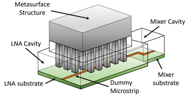
Fig. 3. Representation of the cavities enclosing the amplifier and mixer. The lid containing the artificial magnetic wall is placed above the amplifier he microstrip line includes a bend, only within the mixer cavity, to coincide with the input and output of the amplifier and mixer MMICs, respectively.
