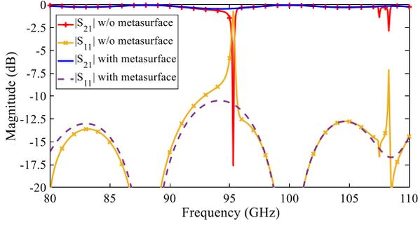
Fig. 1. Simulated  $|S_{21}|$  and  $|S_{11}|$  parameters of a transmission line inside the LNA and mixer cavities. Simulations were performed with and without the PMC metasurface.
