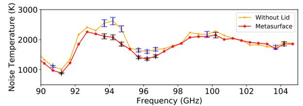
Fig. 6. Measured noise temperature with the top lid removed and the BoN structure. These measurements were made with a fixed IF frequency of 200 MHz and an integrated spectrum of 100 MHz. Error bars at  $1\sigma$  are shown in relevant points [16].
