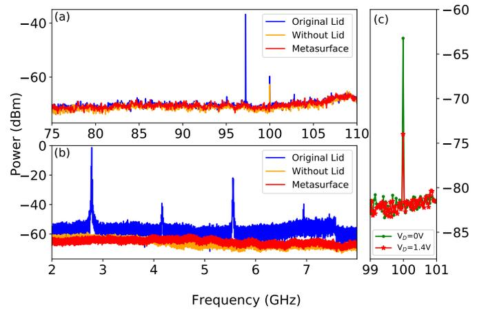
Fig. 5. Power spectrum measurements. (a) RF port of the module. (b) IF port of the module. (c) LO Leakage measurement at the RF input using the metasurface and with two LNA bias settings.
