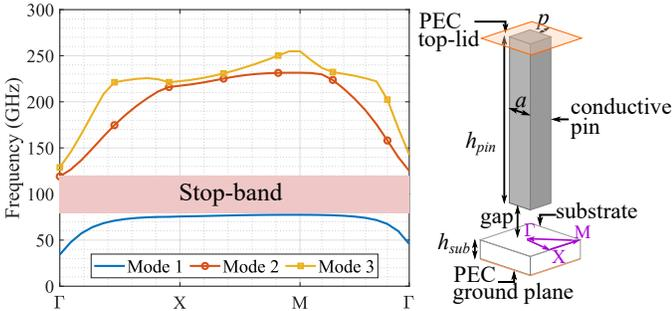
Fig. 2. Dispersion diagram of the proposed structure. Design parameters of the unit cell are  $p = 0.105$  mm,  $h_{pin} = 0.9$  mm,  $gap = 0.2$  mm and  $a = 0.15$  mm.
