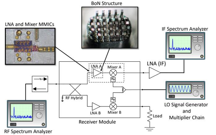
Fig. 4. Diagram of the setup used to measure the instability of the receiver at the RF and IF ports, simultaneously. Two spectrum analyzers were used, an Agilent PXA Signal Analyzer N9030A with a W-Band waveguide harmonic mixer and an Agilent CXA Signal Analyzer N9000A. The insets show the fabricated BoN structure and the LNA and mixer MMICs, respectively.
