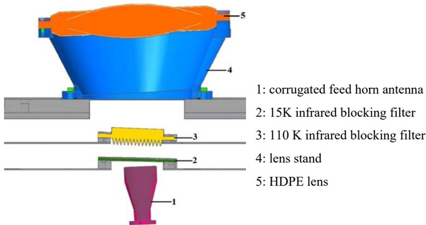
Figure 4. Layout of the ALMA Band-1 optics configuration.
