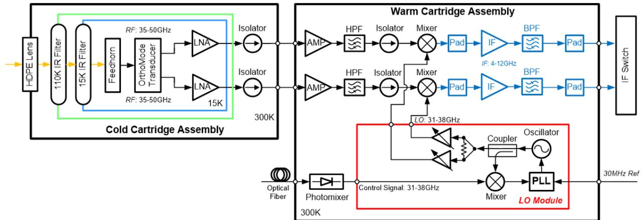
Figure 1. Block diagram of the ALMA band-1 receiver.
