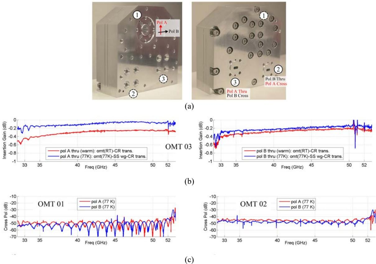
Figure 8. The orthomode transducer for ALMA Band-1, (a) layout of the OMT, (b) measured performance of insertion gain at 300K and 77K, (c) measured performance of cross-polarization at 77K.
