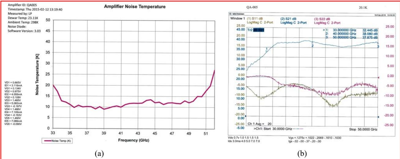
Figure 9. measured results of the 32 – 52 GHz 5-stage InP HEMT hybrid cryogenic low-noise amplifier (CLNA) for preproduction, (a) the noise temperature, (b) the scattering parameters.
