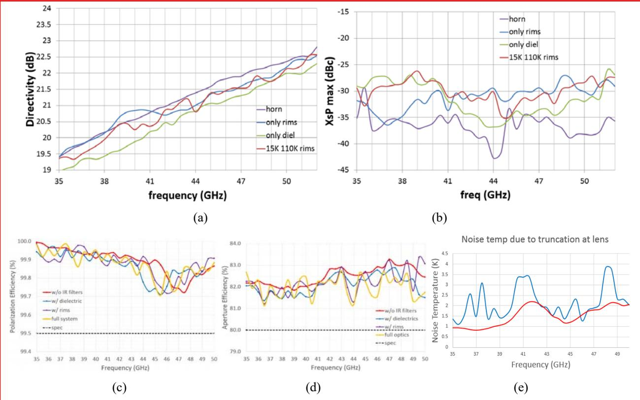
Figure 5. the simulated effects of the truncation and impedance coupling effect due to small IF blocking filter apertures and very small distance to horn antenna, (a) directivity, (b) cross-polarization, (c) polarization efficiency, (d) aperture efficiency, (e) increment of the receiver noise temperature.
