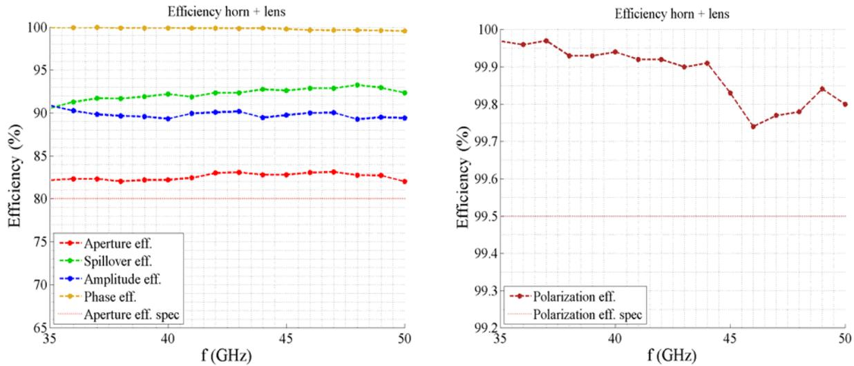
Figure 3. Simulated results of (left) aperture efficiency, spillover efficiency, amplitude efficiency and phase efficiency of the ALMA Band-1 optics lens-horn configuration, and (right) polarization efficiency. Please note the effects of the 110 and 15K IR blocking filters are not included in this simulation.
