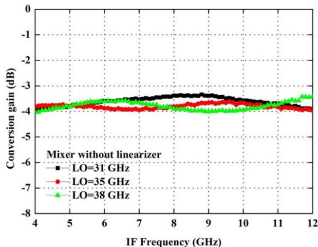
Figure 11. Conversion gain of the 70-nm MHEMT cascode mixers
