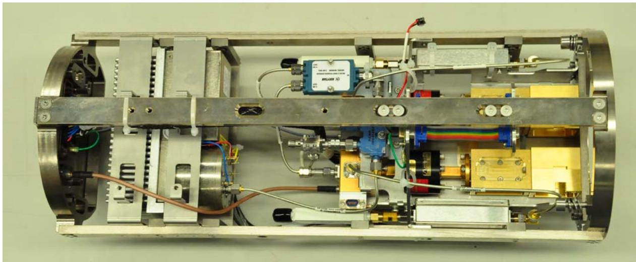
Figure 10. The layout of warm cartridge assembly for ALMA Band-1 receiver.
