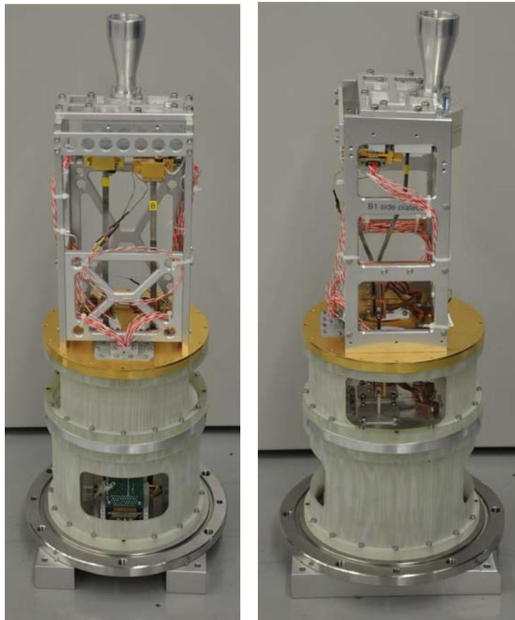
Figure 7. Prototype Cold Cartridge Assembly for ALMA Band-1 receiver
