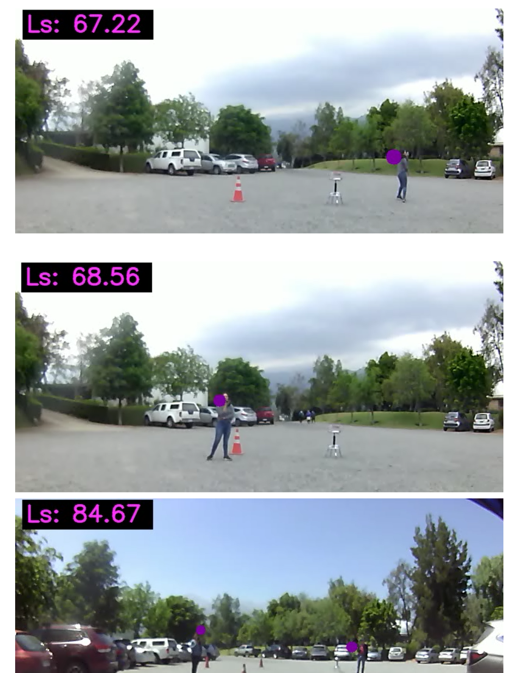
Fig. 7: Examples of the Radiovision GUI. The optical image is obtained from the camera, while the purple markers correspond to the estimates of the phone positions.
