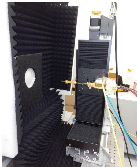
Figure 5. Near-field beam-pattern measurement system. (a) Schematics. (b) Front and back views.
