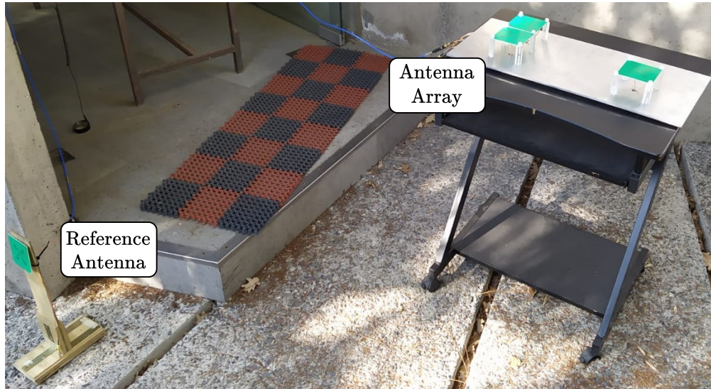
Figure 6.8: Antennas configuration to take measurements.
