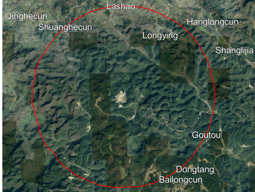
Figure 2.3: Restriction zone of the RQZ established around FAST telescope, the circumference has a radius of 5 km.
