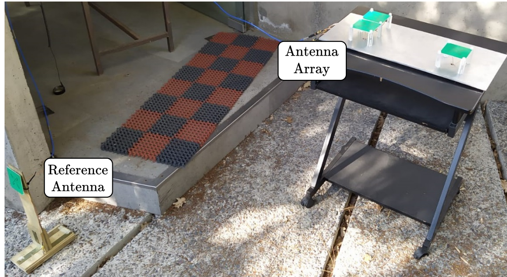
Figure 6.8: Antennas configuration to take measurements.
