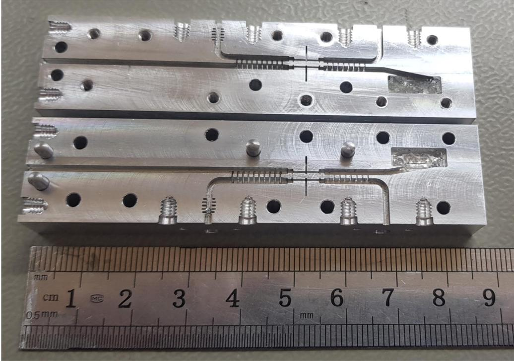
Figure 5.9: Picture of the constructed split-block diplexer.
