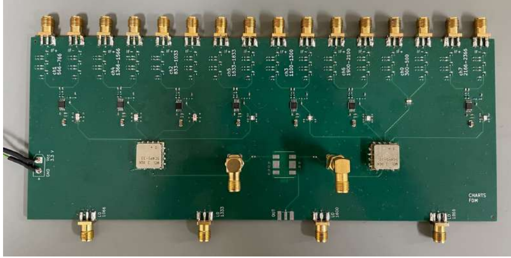
Figure 4.8: Differential FDM design and implementation. The PCB was manufactured by JLCPCB and soldered in the MWL laboratory. The lines were designed as microstrips to better adjust to the LC components of the custom bandpass filter and matching network of the mixer. An auxiliary debugging SMA output was added to the design after the four-way combiners. This connection was added to measure the response of the FDM in case the combiners did not work.
