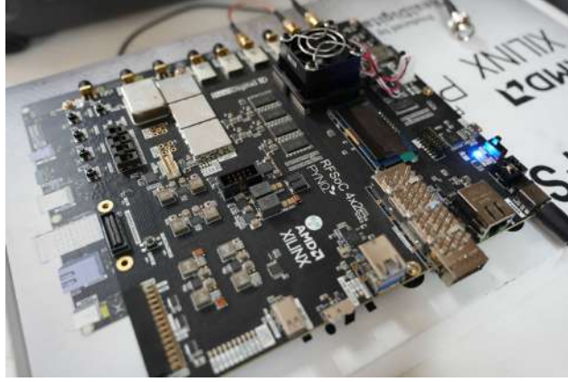
Figure 2.23: One of CHARTS RFSoc 4x2. The board was used for testing and to generate the LOs.
