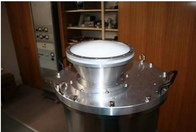
**Figure 46.** *The constructed HDPE lens mounted in top of the test cryostat for the ALMA Band1 prototype receiver.*
