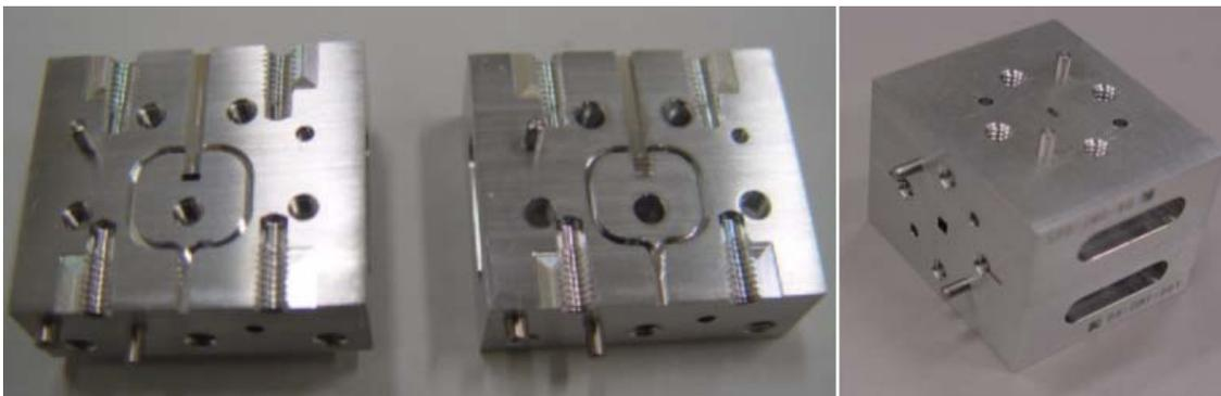
**Figure 21.** Asayama’s Band-4 125--16-GHz OMT showing the two CNC machined split blocks (left picture) and the final assembled device (right picture) [64].
