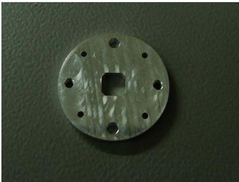
**Figure 89.** The constructed square-to-circular waveguide transition that it will be used to connect the horn with the OMT. It height is of 2.21 mm the radius of the octagonal aperture varies between 2.69 to 3.21 mm.
