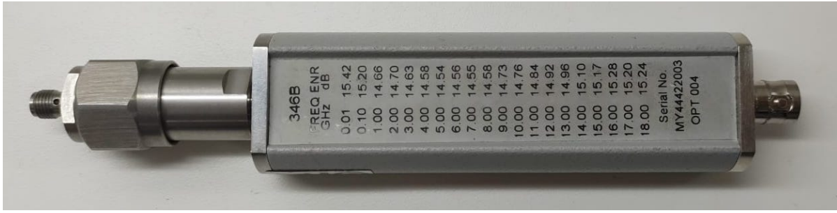
Figure 3.15: Agilent Noise Source 346B [33] back view
