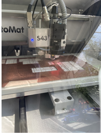
(a) Mechanic LPKF drilling process.
