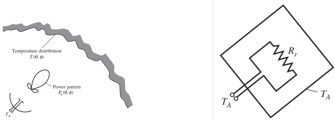
Figure 1.2: (a) The antenna is receiving noise from various directions, represented by the coordinates (\theta, \phi) , resulting in an established antenna temperature denoted as T_A . (b) This illustrates the equivalent model. Figures adapted from Stutzman & Thiele 2012, Ch. 4, p. 104.
