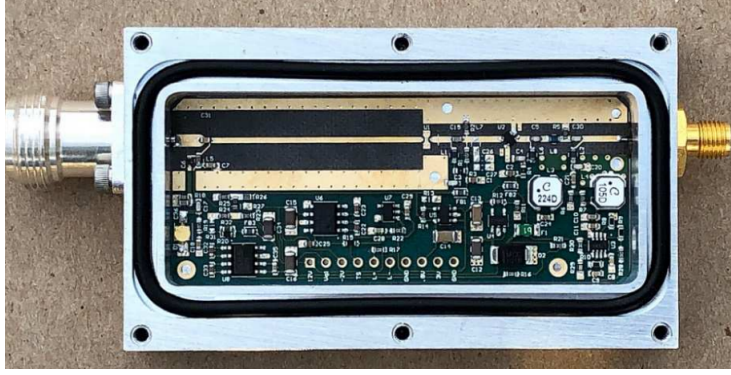
Figure 1.8: LNA design used in the GRex project. Extracted from Weinreb & Shi 2021.
