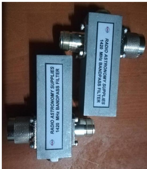
Figure 5.22: Radio Astronomy Supplies bandpass filters.
