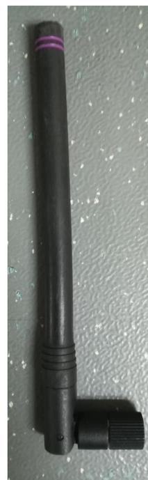
Figure 5.18: Linx 1.4GHz omnidirectional dipole antenna used as reference antenna. Datasheet: <https://bit.ly/2I7JDx9>.
