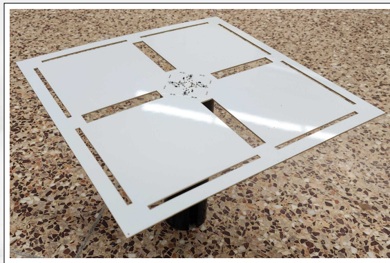
Figure: Differential antenna 300–500 MHz.
