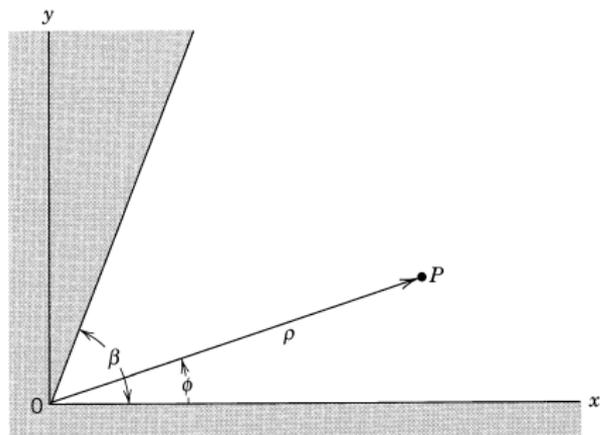
$$\nabla^2 \Phi = \frac{\partial^2 \Phi}{\partial \rho^2} + \frac{1}{\rho} \frac{\partial \Phi}{\partial \rho} + \frac{1}{\rho^2} \frac{\partial^2 \Phi}{\partial \phi^2} = 0.$$
